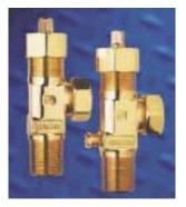
Chlorine valves are made in strict compliance with the standards and specifications of the Chlorine Institute. Valve bodies are forged from corrosion-resistant aluminum silicon bronze alloy "B". Strong, chlorine-compatible Monel® stems are used for long valve service with stem seal packing recognized by the Chlorine Institute. Brass outlet caps with teflon® inserts are included for outlet thread protection. Valves come is two models:
