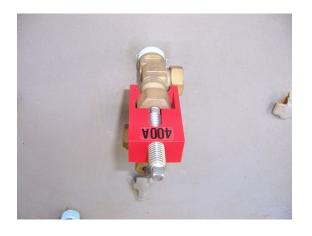
Stripped Valve Stem Clamping Device:
